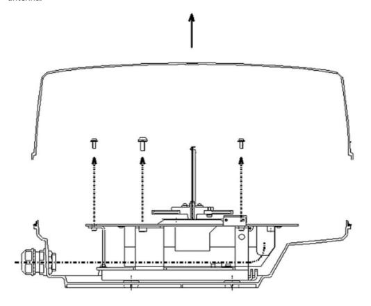
Carefully lift the main unit and stand it upright in the slot on the scanner casing:
